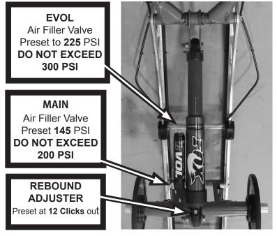
The FLOAT 3 EVOL R Reservoir is positioned to the left side of the vehicle with the Rebound Adjuster facing up. The Rebound Adjuster has a total of 24 clicks. Start counting clicks from the adjusters most clockwise limit.
