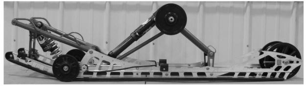
Install the rear suspension. Torque all bolts and mounting hardware to the manufacturer's specifications. Adjust the track tension to the manufacturer's specifications. Air pressures should always be set at the ambient air temperature anticipated during riding conditions.
