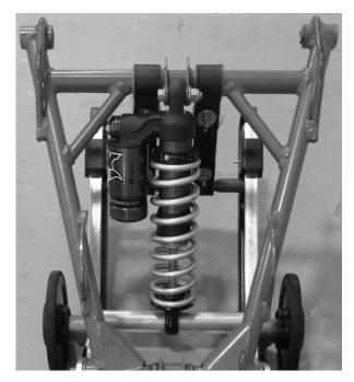
ZERO C2 Low and High Speed Adjusters (DSC) are set at 12 clicks out from bottom. Each has a total of 24 clicks out from bottom. Use a flat blade screwdriver to adjust low speed compression. Use a 17mm hex socket to adjust the high speed compression. The spring should have 1/4" preload.
