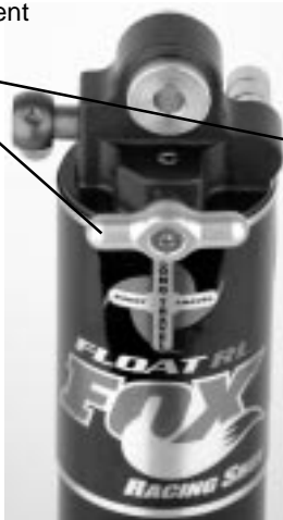
Switch in Short -Travel Position Switch in Long-Travel Position
