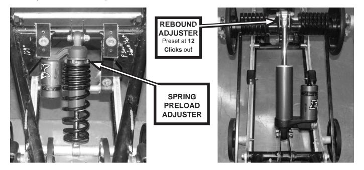
ZERO C2 Low and High Speed Adjusters (DSC) are set at 12 clicks out from bottom. Each has a total of 24 clicks out from bottom. Use a flat blade screwdriver to adjust the low speed compression. Use a 17mm hex socket to adjust the high speed compresssion. Spring has 1/4" preload. ZERO RC2 Reservoir is positioned below the shock with the Rebound Adjuster facing up when connected to the rear arm. Low and High Speed Adjusters (DSC) Each have 24 clicks out from bottom.
