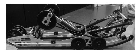
Reset limiter straps and rear spring preload to noted settings. Install the rear suspension. Torque all bolts and mounting hardware to manufacturer's specifications. Adjust the track tension to the manufacturer's specifications.
