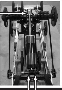
AIR Filler Valve Preset to 50 PSI DO NOT EXCEED 200 PSI
