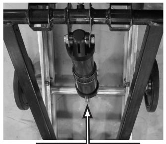
REBOUND ADJUSTER Preset at 12 Clicks out The Rebound Adjuster has a total of 24 clicks, start counting clicks from the adjusters most clockwise limit.
