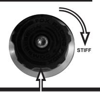
ZERO RC Low Speed Adjusters (LSC) are set at 12 clicks out from bottom. The LSC has a total of 24 clicks. Start counting clicks from the adjusters most clockwise limit.
