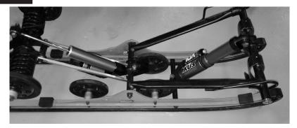
Install the rear suspension. Torque all bolts and mounting hardware to the manufacturer's specifications. Adjust the track tension to the manufacturer's specifications.
