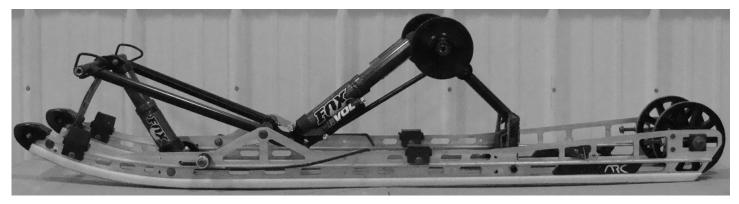
Install the rear suspension. Torque all bolts and mounting hardware to the manufacturer's specifications. Adjust the track tension to the manufacturer's specifications. Air pressures should always be set at the ambient air temperature anticipated during riding conditions.
