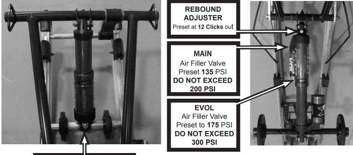
AIR Filler Valve Preset to 50 PSI DO NOT EXCEED 200 PSI Position the EVOL chamber to the left side of vehicle with the Rebound Adjuster facing up. Position the DSC to the right side of the vehicle. The Dual Speed Compression adjuster is set at 12/12. All Adjusters have a total of 24 clicks out from bottom. Start counting clicks from the adjusters most clockwise limit.
