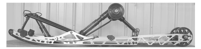
Install the rear suspension. Torque all bolts and mounting hardware to the manufacturer's specifications. Adjust the track tension to the manufacturer's specifications. Air pressures should always be set at the ambient air temperature anticipated during riding conditions.
