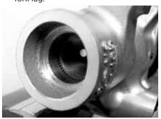
10 Compress the fork so the MX-C damping rod is sticking out of the bottom of the fork lug. Install a fork spring clip tool (e.g., PN 398-00-092) between the top of the lock nut and the fork lower lug. This will hold the damping rod in the compressed state while installing the rebound adjuster onto the rod.
