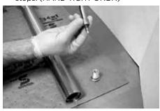
4 Slide the spring tube onto the FOX MX-C Cartridge with the steel spring seat facing spring side.
