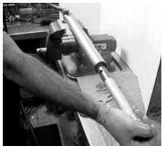
14 Check for proper spring preload. Hold the cartridge to full extension and check to see if you have proper spring preload. You should have zero gap (free space)! If you have any gap, you will need to add more preload washers (see steps 5 & 6).
