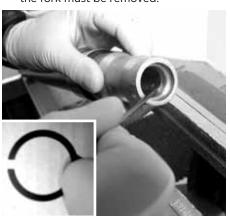
2 Clean and inspect all parts, install new fork seals and bushings. Refer to the fork service manual for your motorcycle, for proper installation
