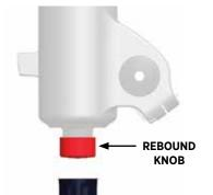
**Rebound** controls the rate of speed at which the fork extends after compressing.
