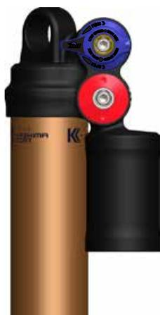
**The 2-position lever** is useful to make on-the-fly adjustments to control shock performance, and is intended to be adjusted throughout the ride. The Open mode utilizes your standard HSC/LSC, preset high- and low-speed compression settings. The preset high- and low-speed compression adjustments only have an affect on compression damping when the lever is in the OPEN position. The FIRM mode has a very firm low-speed compression setting and is useful for climbing and sprinting.
