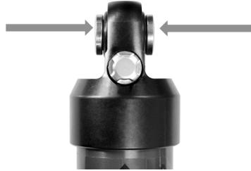
**WARNING:** Contact FOX if these reducers do not fit correctly. Correct shock mounting is critical for correct operation and for your safety.
