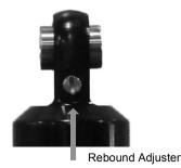
The Rebound Adjust feature on your FLOAT 3 EVOL RC2 shocks gives you the ability to externally adjust the shock rebound damping. Adjustments are made by turning Rebound Adjuster using a Quarter or a small flat-bladed screwdriver to turn adjuster on the Air Sleeve Body Cap located on the end of the shock absorber.
