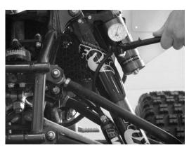
**STEP 2** Thread the pump onto the EVOL air filler valve until it is fully seated and air pressure registers on the pumps high pressure scale.
