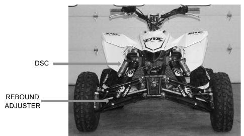
STEP 1 Install shock absorbers as per above photo with DSC mounted to the top with the DSC on outboard side of ATV.
