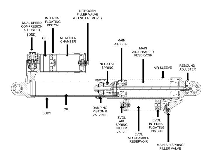
FLOAT 3 EVOL RC2 shocks are built using 6061-T6 aluminum for light weight and strength. The chromed damper shaft is super-finished for low friction and long seal life. All of the seals and wipers are engineered specifically for FLOAT 3 EVOL RC2. The Air Sleeve and Reservoir are Genuine Kashima coated for reduced friction and long seal life. The damper shaft and seals are contained within the air sleeve, protecting them from debris, dirt and water.
