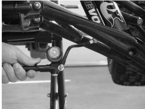
**STEP 4** Thread the pump onto the MAIN air filler valve until it is fully seated and air pressure registers on the pumps low pressure scale.
