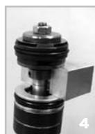
**NOTE:** You will need to compress the coil spring in order to install the shaft clamps between the free piston and the compression piston backup plate.
