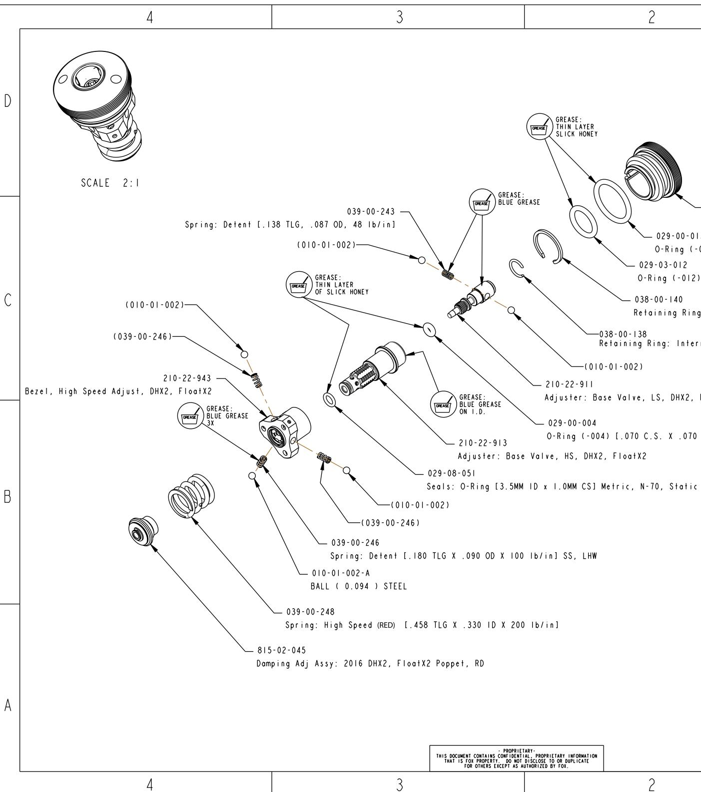
\_ 234-04-874 Cartridge, Housing Cap, RD, DHX2, FloatX2 029-00-015 O-Ring (-015) [.070 C.S. X .551 ID] 029-03-012 O-Ring (-012) [.070 C.S. X .364 ID] 038-00-140 Retaining Ring: Internal, Smalley XAH-50, 302 SS -038-00-138 Retaining Ring: Internal, Round Wire [.031 Wire OD, .245 free ID] Adjuster: Base Valve, LS, DHX2, FloatX2 O-Ring (-004) [.070 C.S. X .070 ID]
