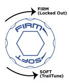
The BRAIN shocks is equipped with FOX BrainFade suspension technology. BrainFade allows you to dial in your shock to match riding conditions, from a fully locked out suspension to soft TrailTune, which provides a stable yet supple platform that soaks up bumps but keeps suspension bob to a minimum during hard pedaling.
