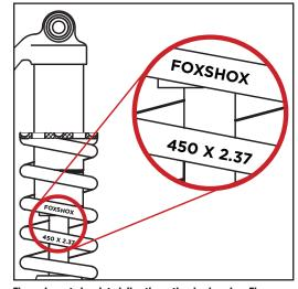
The spring rate is printed directly on the shock spring. The spring above has a 450-lb/in spring rate with 2.37" of travel.
