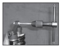
Inserting Bolt Extractor Tool Into Reducer
