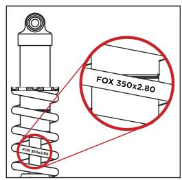
The spring rate is printed directly on the shock spring. The rate above denotes a 350-lb/in spring rate with 2.80" of travel.
