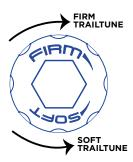
The BRAIN REMOTE shock is equipped with FOX BrainFade suspension technology. BrainFade allows you to dial in your shock to match riding conditions, from firm TrailTune to soft TrailTune, which provides a stable yet supple platform that soaks up bumps but keeps suspension bob to a minimum during hard pedaling.
