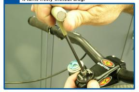
With a 5mm hex key socket and torque wrench, torque all 3 upper crown bolts to 65 in-lb (734 N-cm). DO NOT OVERTORQUE the crown bolts.
