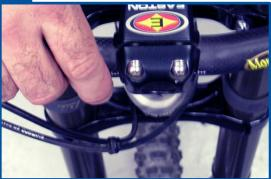
Adjust the steering stop bumpers to the proper height and angle on the upper tubes so that you have maximum turning angle. Depending on the shape and size of the frame tubes, you may need to use the thicker part of the bumper.
