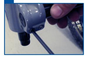
Lightly lube the axle with grease. Install the front wheel into the dropouts, then insert the axle into the lower leg, threading the axle through the wheel.
