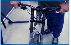
Torque the handlebar pinch bolts to the manufacturer's specifications.
