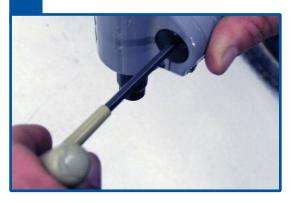
Using a 5mm hex key socket and torque wrench, torque the axle to 19 in-lb. (215 N-cm).
