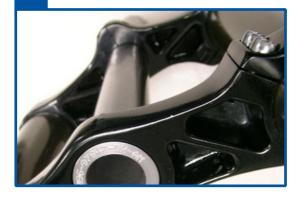
Install the headset spacers (if required) and stem on the steerer and lightly tighten the stem pinch bolt(s). Again, there is no need to overtighten.
