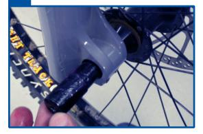
Alternately tighten the left-side M5 pinch bolts until an even torque of 19 in-lb. (215 N-cm) is obtained. DO NOT OVERTORQUE the pinch bolts.
