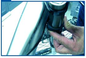
Route the disc brake hose from the caliper through the inside of the lower leg and through the supplied disc brake hose guide. Assemble parts in the orientation shown.
