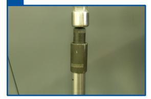
Install the FOX 40 onto the bicycle with all of the headset parts and upper crown. Use a plastic mallet, if needed, to tap parts into place.
