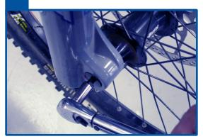
Compress the fork on the bike a couple of times to let the right side of the dropout settle into its low-friction point. Alternately tighten the right-side M5 pinch bolts until an even torque of 19 in-lb. (215 N-cm) is obtained. DO NOT OVERTORQUE the pinch bolts.
