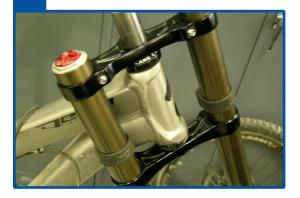
Verify that the upper tubes are 176.4mm above the top surface of the lower crown. Use a pen and mark the upper tubes at the upper edge of the lower crown.
