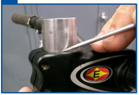
Using a 5mm hex key wrench, remove the upper crown and fork from the bicycle. Using a 5mm hex key, remove the lower crown assembly from the upper tubes. Cut the steerer 3mm below the scribed line on the steerer. This allows room for the stem cap to lightly tension the headset and eliminate any play.
