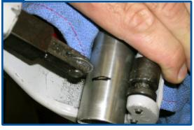
With a star-fangled nut installation tool, install the star-fangled nut into the steerer to the headset manufacturer's specified depth.
