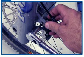
Using a 2.5mm hex socket and torque wrench, torque the disc brake hose guide fastener to 8 in-lb. (90 N-cm).
