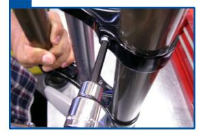
To install the front wheel, loosen the 4 axle pinch bolts on the lower leg with a 5mm hex key.
