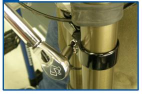
Install spacers (if necessary), stem, stem cap and M6 stem cap bolt. With all three upper crown bolts loosened, lightly tighten the headset stem cap bolt to remove play in the system so that it turns freely without drag.
