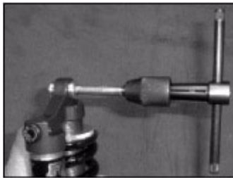
Inserting Bolt Extractor Tool Into Reducer
