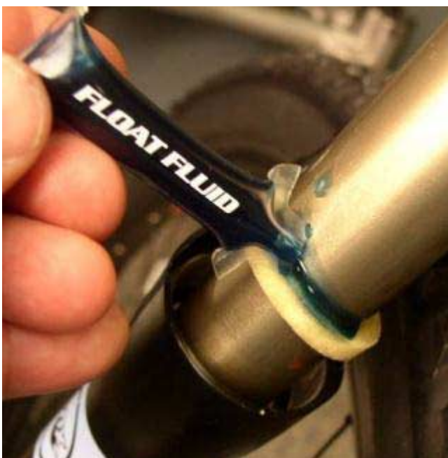
12. Push foam ring down into dust wiper seal gland bore
