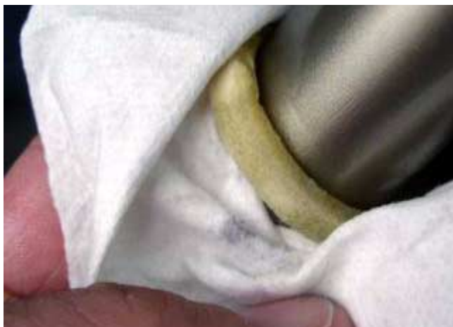
11. Apply FLOAT Fluid to the foam ring 1/2 of a 5 cc pillow pack.
