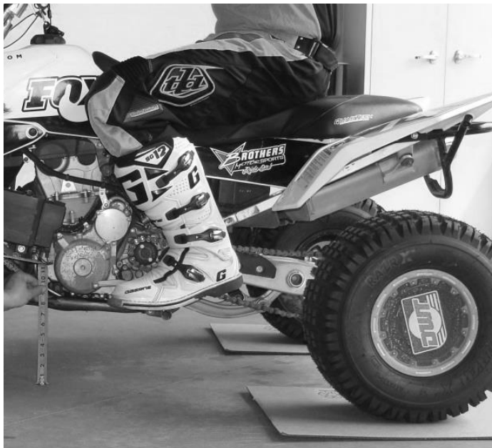
Measure from the ground to the bottom of the frame just below front motor mount.
