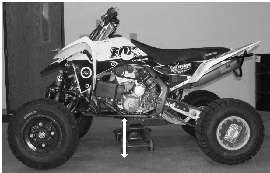
Full extension measuring point.
