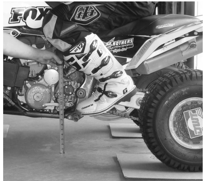
Measure from the ground to the bottom of the frame just ahead of the rear foot peg.
