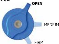
The **3-position lever** is useful to make on-the-fly adjustments to control fork performance under significant changes in terrain, and is intended to be adjusted throughout the ride.
