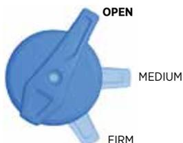
The **3-Position Micro Adjust** lever is useful to make on-the-fly adjustments to control fork performance. Use the positions between the OPEN, MEDIUM, and FIRM modes to fine-tune your compression damping.
