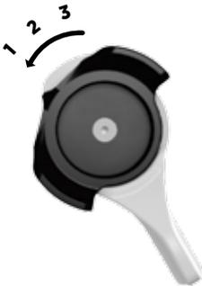
**Open mode adjust** is useful to control shock performance during rider weight shifts, G-outs, and slow inputs.
