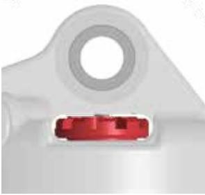
**Rebound** controls the rate of speed at which the shock extends after compressing.
