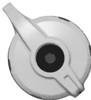
**Open mode adjust** is useful to control shock performance during rider weight shifts, G-outs, and slow inputs.
