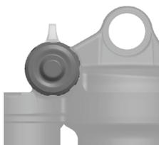
**Rebound** controls the rate of speed at which the shock extends after compressing.
