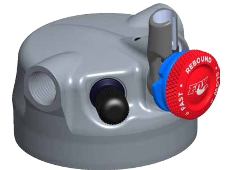
808-17-318-KIT Eyelet Assy: 2017, Float DPS Remote up, PTL, Trunnion, LV 808-17-338-KIT Eyelet Assy: 2018, FLOAT DPS Remote up, PTU, Trunnion, LV
