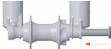
**⚠ WARNING:** Use hand pressure only. Never use any tool to tighten the 15QR levers onto the lower legs. Over-tightening the levers can damage the axle or fork dropouts, leading to a sudden failure with one or more of these components, resulting in **SERIOUS INJURY OR DEATH**.
