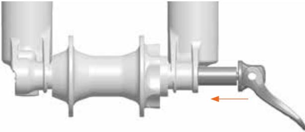
3. Turn the axle clockwise 5-6 complete turns into the axle nut.
