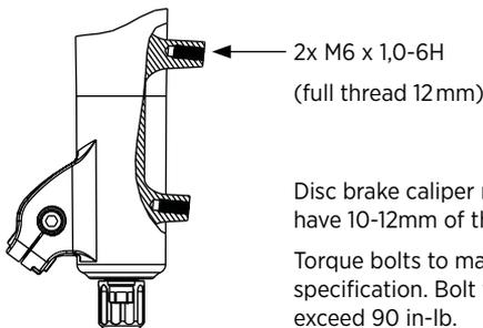
Disc brake caliper mount bolts must have 10-12mm of thread engagement.
