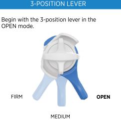
The **3-position** lever is useful to make on-the-fly adjustments to control shock performance under significant changes in terrain, and is intended to be adjusted throughout the ride.
