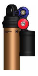
The 2-position lever is useful to make on-the-fly adjustments to control shock performance, and is intended to be adjusted throughout the ride. The Open mode utilizes your standard HSC/LSC, preset high- and low-speed compression settings. The preset high- and low-speed compression adjustments only have an affect on compression damping when the lever is in the OPEN position. The FIRM mode has a very firm low-speed compression setting and is useful for climbing and sprinting.
