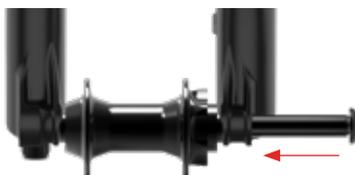
**⚠ WARNING:** Use hand pressure only. Never use any tool to tighten the 15QR levers onto the lower legs. Over-tightening the levers can damage the axle or fork dropouts, leading to a sudden failure with one or more of these components, resulting in **SERIOUS INJURY OR DEATH.**
