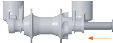
**⚠ WARNING:** Use hand pressure only. Never use any tool to tighten the 15QR levers onto the lower legs. Over-tightening the levers can damage the axle or fork dropouts, leading to a sudden failure with one or more of these components, resulting in **SERIOUS INJURY OR DEATH.**
