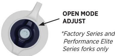
**\*OPEN mode adjust** is useful to control fork performance under rider weight shifts, G-outs, and slow inputs.
