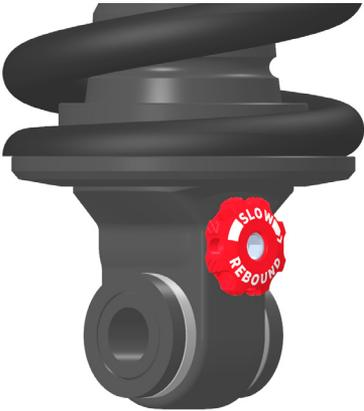
Rebound controls how fast the shock extends after compressing. Turning your rebound knob clockwise slows down rebound. Turning your rebound knob counter-clockwise speeds up rebound.
