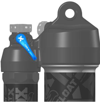
The **2-position lever** is useful to make on-the-fly adjustments to control shock performance, and is intended to be adjusted throughout the ride. The OPEN mode utilizes your standard LSC, preset low-speed compression setting. The preset low-speed compression adjustment only has an affect on compression damping when the lever is in the OPEN position. The FIRM mode has a very firm low-speed compression setting and is useful for climbing and sprinting.
