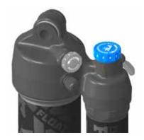
The **Low-Speed Compression** knob allows for changes in low-speed compression damping. Turn the knob clockwise to increase compression damping and counter-clockwise to decrease compression damping
