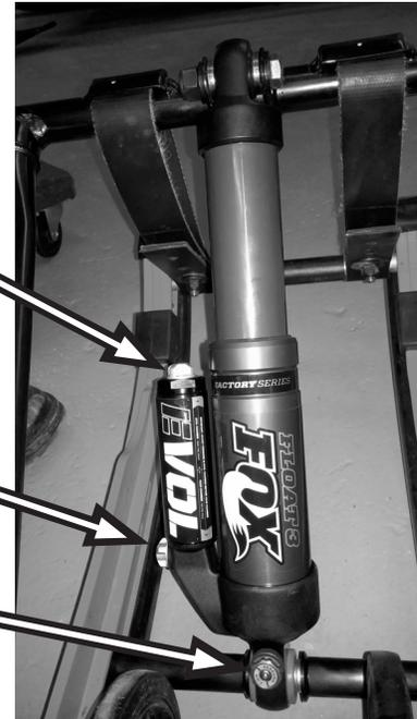
Assemble the upper rear pull rod pivot using the supplied bolt 100mm long and quantity (2) of the supplied washer .060" thick. Put the washer between the pull rod and the rear arm pivot. Quantity (1) per side as arrows indicate above.
