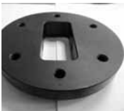
Fig. 3: Correct bolt pattern has no dot marking
