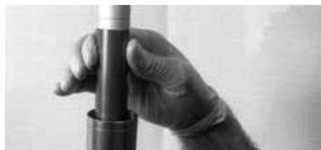
**15** Fill the outer chamber of the fork with a premium 5 wt. racing fork fluid. The recommended oil volume for the Showa fork is 170 cc. The Kayaba fork oil volume is 160 cc. See the FOX MX-C owner's manual for fork oil volume tuning.
