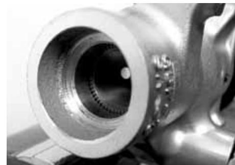
**10** Compress the fork so the MX-C damping rod is sticking out of the bottom of the fork lug. Install a fork spring clip tool (e.g., PN 398-00-092) between the top of the lock nut and the fork lower lug. This will hold the damping rod in the compressed state while installing the rebound adjuster onto the rod.
