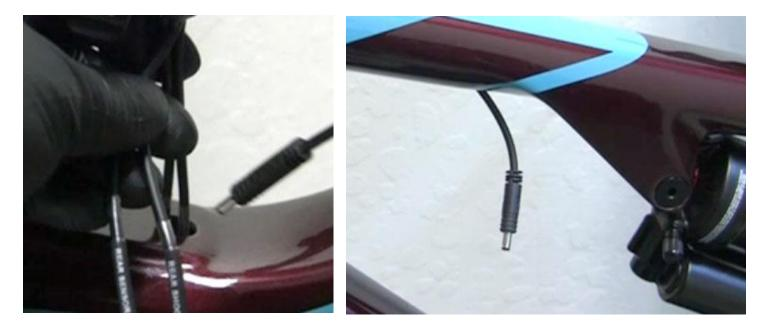
8. Route the LIVE Valve Rear Shock Cable to the rear shock as close to the frame as possible and through any shock mounting tabs that leave enough clearance for shock rotation without contacting the cable.
