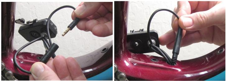
11. As different frames will have different Rear Sensor Cable routing, attach the Rear Sensor Cable to existing brake housing using the provided LIVE Valve MTB Cable to Brake Housing Clips. Install the LIVE Valve cable into the clip first, then install the clip with LIVE Valve cable onto the Brake Housing.
