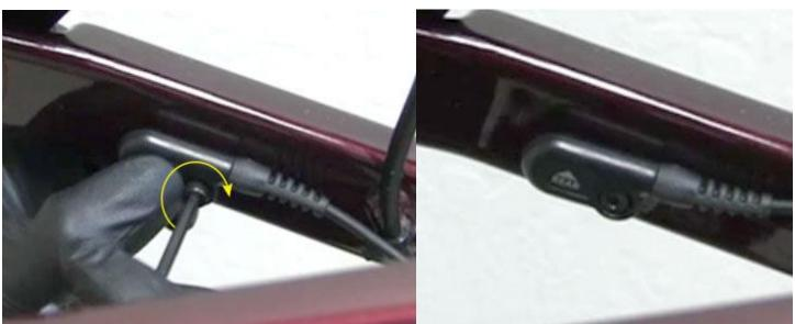
3. Check to verify that the rear disc brake does not contact the Rear Sensor or Rear Sensor Cable.
