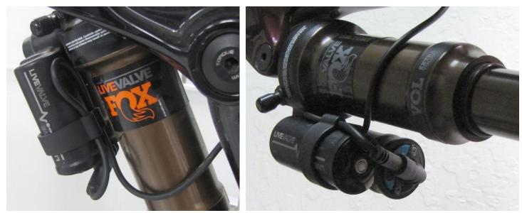
Cable to the Rear Shock Cable port in the LIVE Valve Rear Shock reservoir end.
