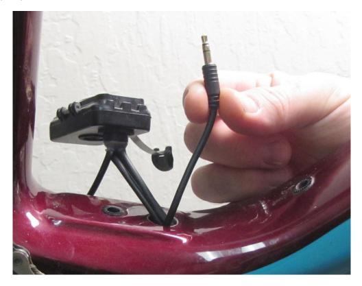
10. Connect the cable from the LIVE Valve Rear Sensor to the LIVE Valve Rear Sensor Cable from the Controller. This connector has a noticeable "click" when mated properly. Push the cable connection and any excess cable into the frame.
