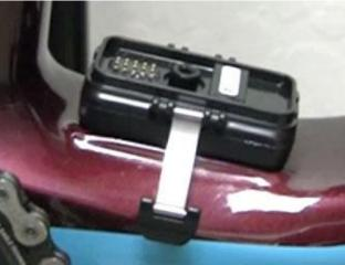
14. Install the LIVE Valve MTB Controller Cover by orienting it so the tabs of the cover interface with the notches in the controller. Attach the two buckles into the grooves of the cover then click them closed.
