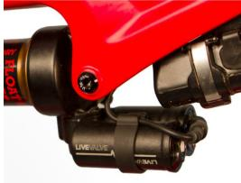
• For frames with the Rear Shock Cable routing approaching the rear shock from the body end: Install the provided LIVE Valve MTB Cable to Reservoir Clip so the Rear Shock Cable goes through the clip once, turns 180 degrees, then goes through the clip again, creating a strain-relief loop of cable. Connect the Rear Shock
