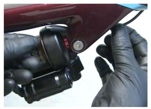
• For frames with Rear Shock Cable routing approaching the rear shock from the reservoir end: Install the provided LIVE Valve MTB Cable to Reservoir Clip so the Rear Shock Cable goes through the clip once then connects to the Rear Shock Cable port in the LIVE Valve Rear Shock reservoir end. Install the clip onto the smaller diameter reservoir with the black end cap (not the reservoir with the LIVE connector and compression adjuster).
