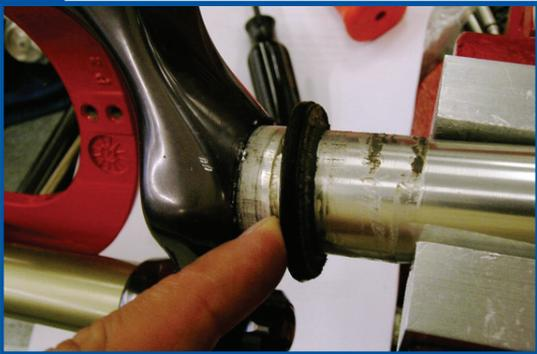
**04** Transfer the measurement from the old fork onto the steerer of your new FOX fork. Use a scribe or marker to mark the cut line. If you are adding spacers to your new setup, add the height of the spacer(s) to the new measurement before cutting.
