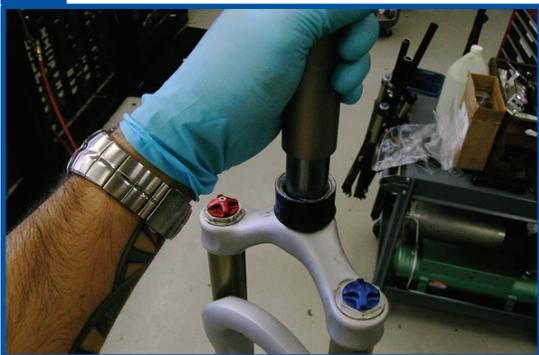
**09** Using a star-fangled nut installation tool, install the supplied star fangled nut. Do not
