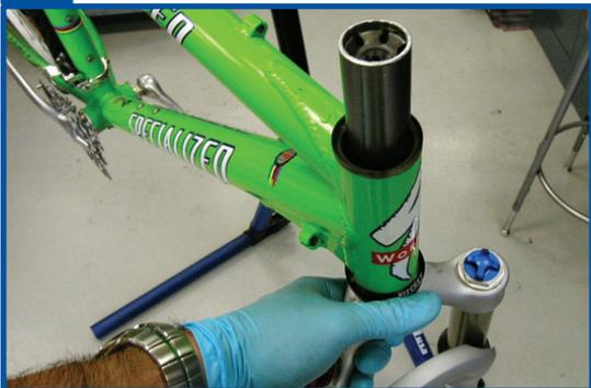
**11** Place the requisite headset parts, spacers and stem onto the steerer tube and tighten bolts to manufacturer's specification. Place the stem cap and stem cap bolt on the stem and torque to manufacturer's specification.
