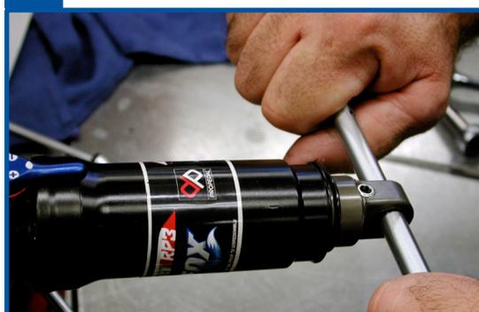
**09** Put on your gloves and place a shop towel through the body eyelet to prevent the air sleeve from coming off. Use a strap wrench to turn the air sleeve counterclockwise. **YOU MAY HEAR A VERY LOUD POP WHEN REMOVING THE AIR SLEEVE!** This is normal on a “stuck down” shock.
