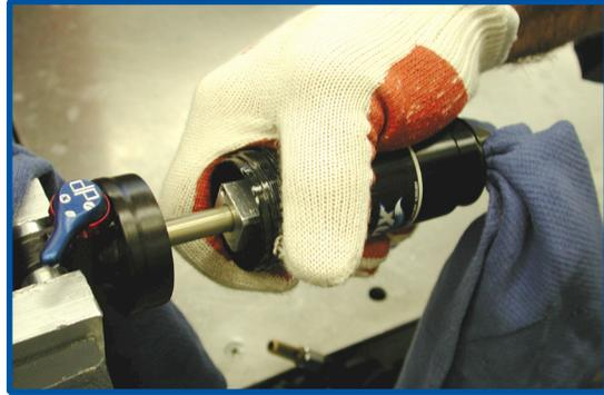
**11** Remove the shop towel from the body eyelet then fully remove the air sleeve.
