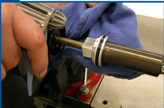
**14** If necessary replace seals and backup rings with new seals and backup rings from the Air Sleeve Rebuild Kit, FOX P/N 803-00-142, as described in the following steps.
