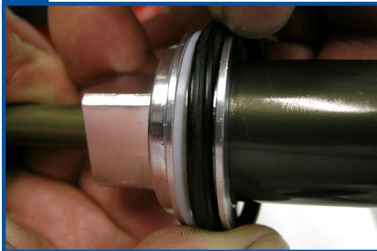
**19** If necessary, replace the shaft eyelet o-ring. Carefully remove the old o-ring using a dental pick. Lightly lubricate the new o-ring before installing it.
