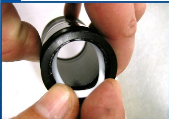
**22** Slide the air sleeve onto the body. Do not screw the air sleeve on at this time.
