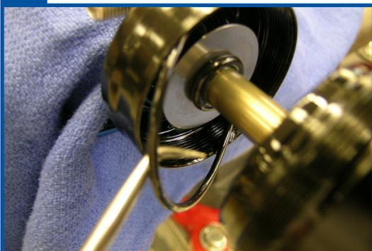
**20** If necessary, remove the air sleeve dust wiper, seal and backup rings. Carefully remove these parts using a dental pick. If you are not removing these parts, skip to step 22.
