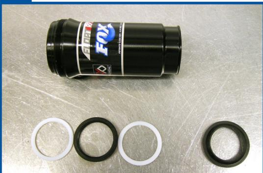
**16** Two shaft eyelet o-rings are supplied with the Air Sleeve Rebuild Kit; a 2000-04 FLOAT rear shock uses the thicker o-ring, the 2005 and newer uses the thinner o-ring.
