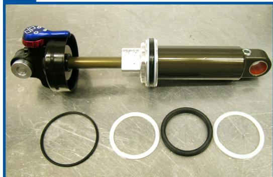
**17** Remove the body seal (quad ring) and two backup rings, being careful not to scratch the inside of the seal gland.
