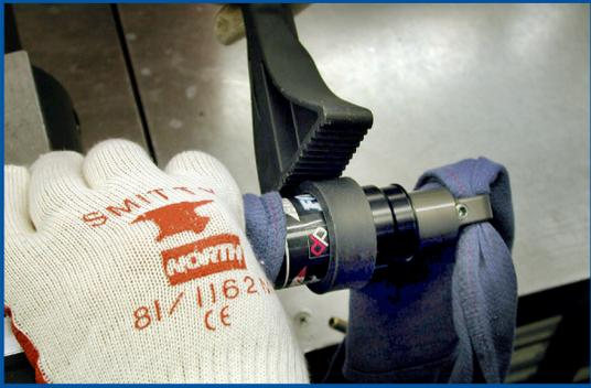
**10** Finish unscrewing the air sleeve by hand and pull it back from the shaft.
