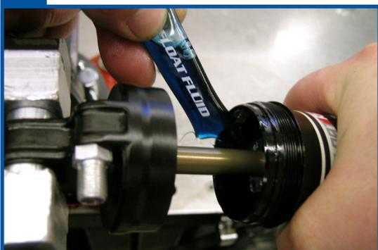
**24** Install the travel indicator o-ring onto the body. Place the reducers (or requisite mounting hardware) back onto the body eyelets.
