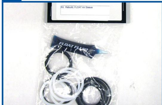
**15** When replacing the air sleeve wiper, seal and backup rings, ensure that they are properly oriented. Lightly lubricate all seals and rings before installing them. Use no more than half of the FLOAT Fluid pillow pack for this entire procedure.
