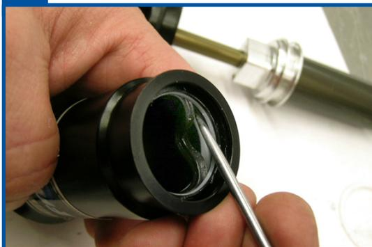
**21** Replace the backup ring, seal, backup ring, and dust wiper into the air sleeve seal glands. Tip: Squeeze the backup ring like a "potato chip," as shown, to facilitate installation.
