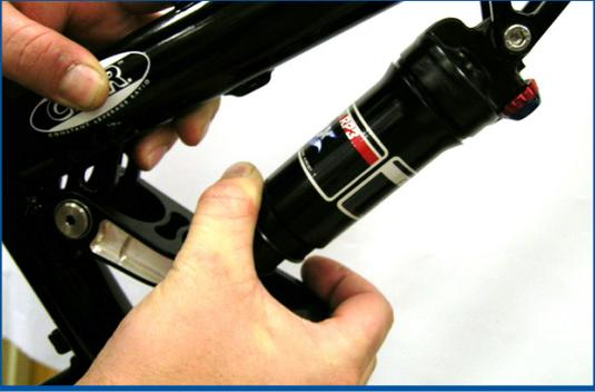
**26** Press down on the bicycle seat to compress the rear suspension. This will make it easier to screw on the air sleeve. Thread the air sleeve by hand until it is tight. **DO NOT** overtighten with a strap wrench or other tool.
