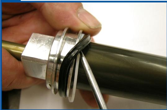
**18** Lightly lubricate the seals and rings before replacing them. Make sure that you use the backup rings with slits. In this order, install a backup ring, body seal (quad ring), then the other backup ring onto the seal gland.
