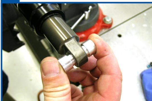
**25** Mount the shock back onto the bicycle using the appropriate mounting hardware. Torque the bolts to the bicycle manufacturer's specifications. Due to frame design, you may have to tighten the air sleeve before re-installing the shock.
