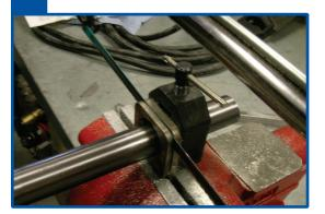
Install the crown race on your FOX fork using a crown race installer tool.
