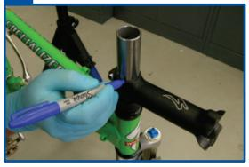
Use a scribe to mark another line 3 mm below the line marked in step #3. THIS IS YOUR CUT LINE. Remember to measure twice, and cut once. If you are not sure, have your fork professionally installed.
