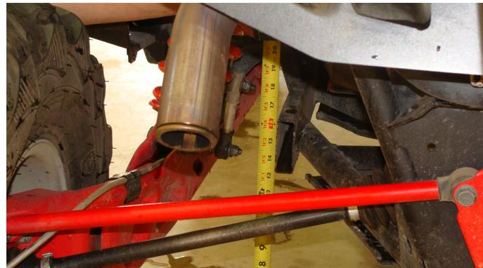
**WARNING:** Do not add excessive amounts of preload into the coil spring. Doing so may result in coil-bind, which could lead to spring failure and potential injury or death. To check coil-bind, put several zip-ties around individual coils. If they break or show contact, there is excessive preload. If you are at maximum preload and need more ride height, contact FOX for a stiffer spring.
